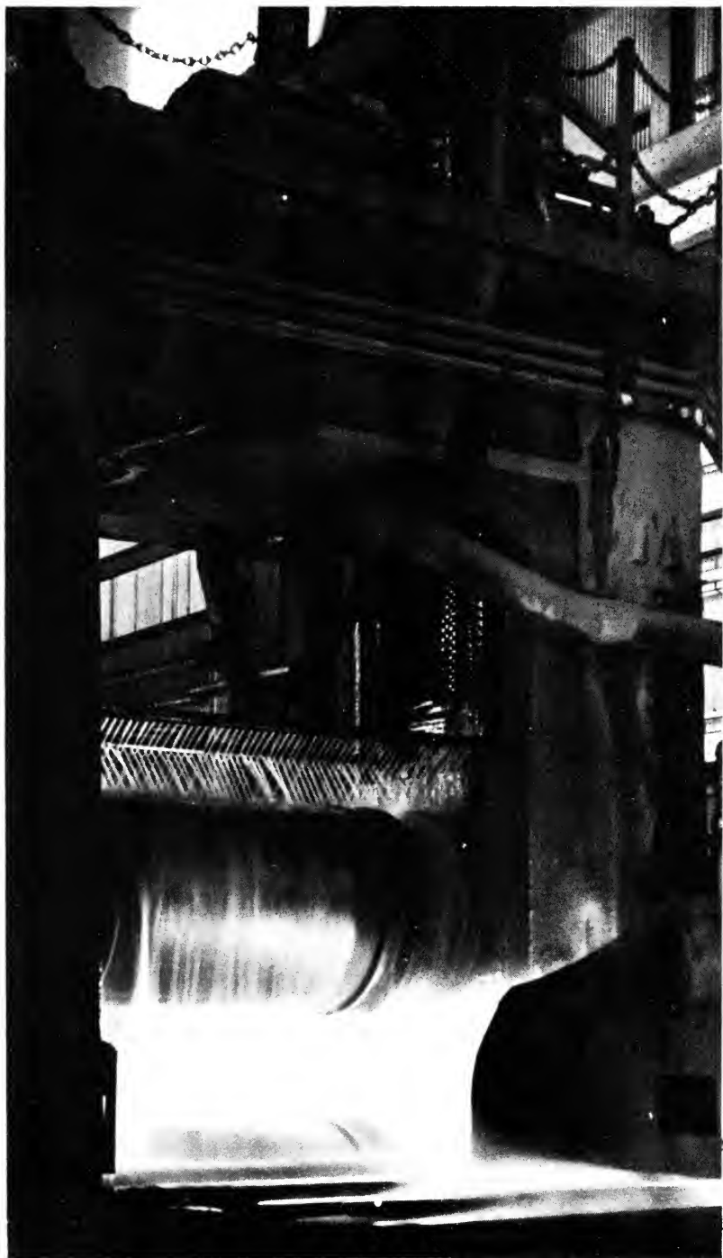
White Hot Steel Ingot Being Rolled into Blocks in Inland Steel Co.
