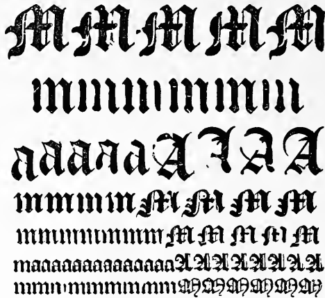
2. Specimens illustrating the variations in the face of type produced by bad casting.
