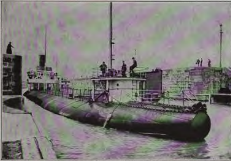
FIG. 10. Modern Lake and Canal Transportation. A whaleback freighter passing through the "Soo" locks in the Sault Ste. Marie canal between Lake Superior and Lake Huron.
