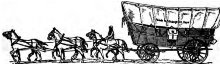
FIG. 14. The Conestoga wagon, the predecessor of the freight car in the Middle Atlantic States
