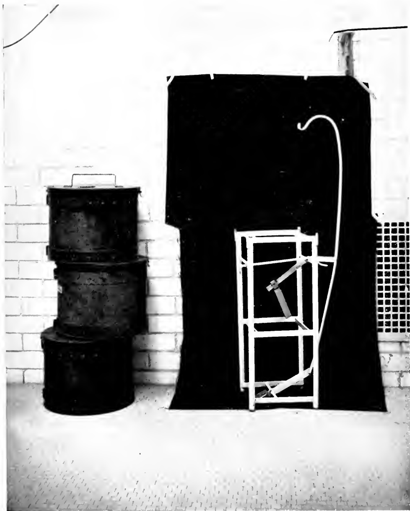
Fig. 4.—Copper canisters for gauzes and draperies. Canister stand with movable balance weight for cover.
