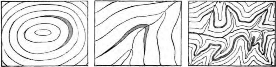
Fig. 27-29.—Behavior of the outcrops of horizontal strata in diverse types of topography.
