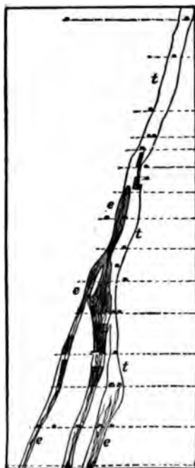
Fig. 157.—Cross-section through the main veins of the Bergmannstrost mine, 70 m. east of the Marien shaft. (Zirkler.) e, ore-carrying; t, barren veins. The dark places have been worked out
