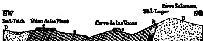
Fig. 50.—Profile through a part of the Rio Tinto ore field. (A. Phillips.) s, clay slate; p, porphyry; k, copper ore bed; e, Pleistocene iron ores.
