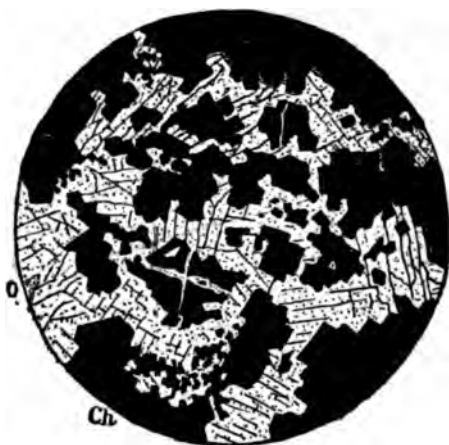
Fig. 7.—chromitiferous olivine rock of Ramberg. (Enlarged 50 times.) o, olivine; ch, chromite.
