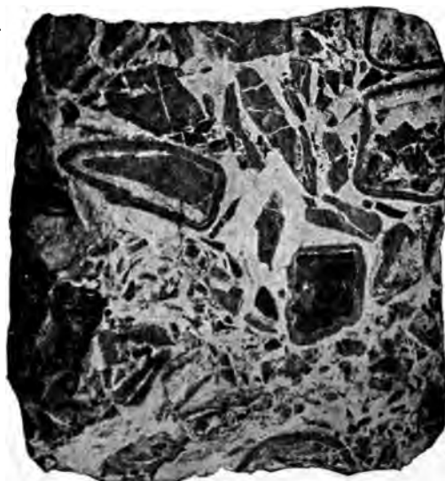
Fig. 134.—Ring ore from the "Ring und Silberschnur" mine in the Harz. (From nature.)
