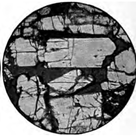
Fig. 19.—Augite crystals (bright) cemented by niccolite (dark); with incident and also transmitted light. (Enlarged 10 times.)
