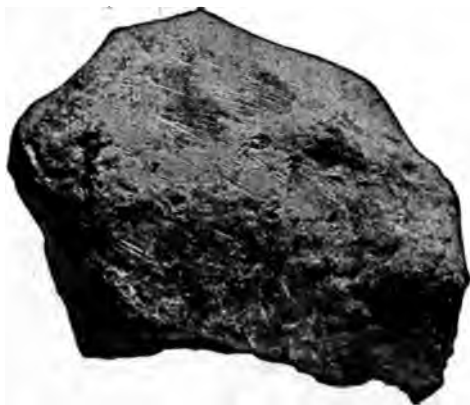
Fig. 90.—A fault cobble with scratches. From Daniel lode on Himmelsfürst. (A part broken off.) (From nature, two-thirds natural size.)
