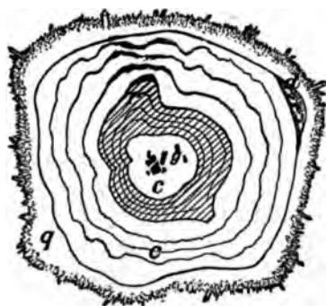
Fig. 140.—Cross-section through a stalactite of Verespatak. (Posepny.) g, gold; c, calcite; r, rhodonite; q, quartz; d, druse.
