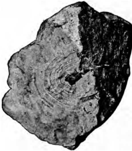
Fig. 132.—Concentric crusts of the Drei Prinzen Spat (a baritic lead vein). (From nature.)
