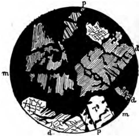
Fig. 14.—Nickel ore of Varallo under the microscope, with fifty-fold enlargement. d, diallage; p, plagioclase (with crossed nicols); m, magnetic pyrite.
