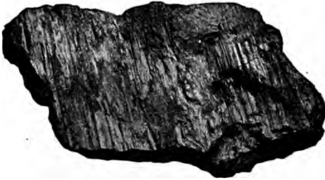
Fig. 96.—Striated surface of galena from Lade des Bundes lode in Himmelsfürst mine. (From nature. One-fifth natural size.)
