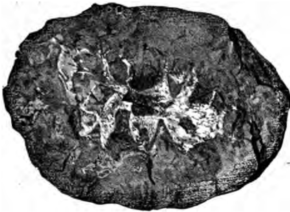
Fig. 37.—Lens of sphaerosiderite from the clay slate of Bocksberg, split longitudinally. (One-fourth natural size.)
