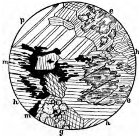
Fig. 15.—Ore-bearing norite from Solum Schurf, northwest of Erteli. (Enlarged 50 times.) e, enstatite; p, plagioclase; h, hornblende; g, garnet; m, magnetic pyrite.
