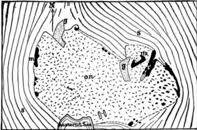
Fig. 8.—Sketch-map of the Erteli mineral region. (Vogt.) s, crystalline schists; on, olivine norite and other varieties of norite; g, granite; m, ore masses.
