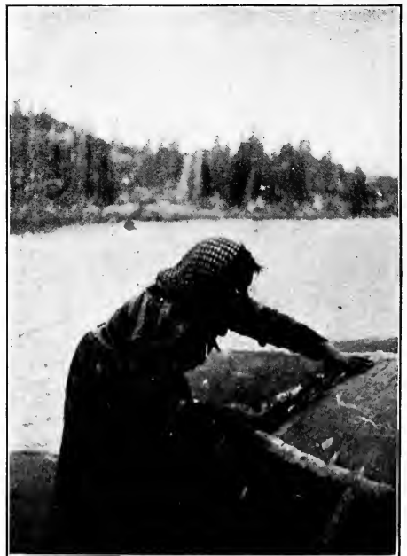
REPAIRING A CANOE. A FIREBRAND AND WHITE SPRUCE GUM ARE USED
