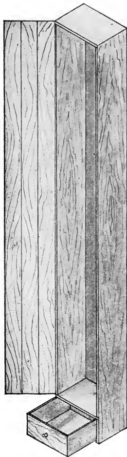
THE CASE FOR HANGING THE ROD WITH THE TACKLE DRAWER AT THE BOTTOM
