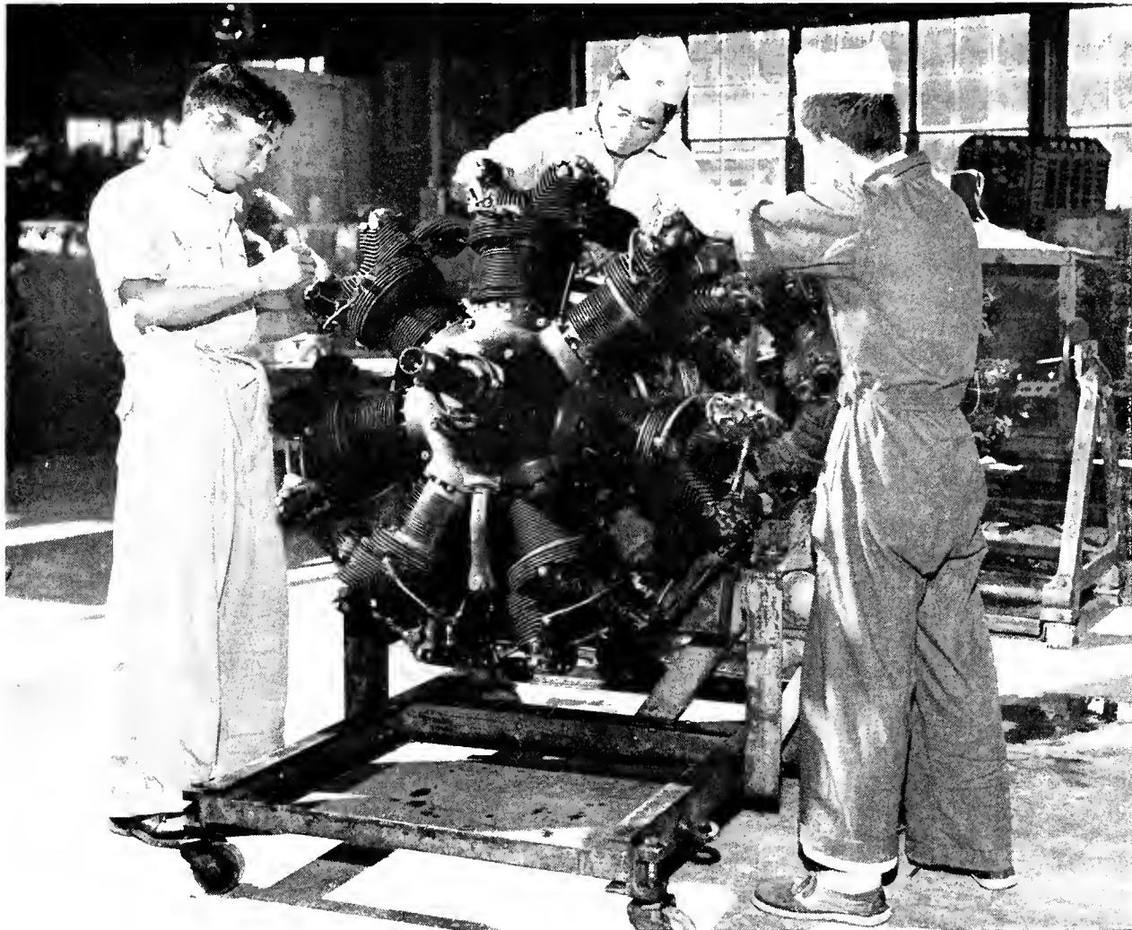
Chinese air force mechanics overhauling a Continental aircraft engine at the Cadet Flying School in Formosa. A United States Military Advisory Group is helping to train the armed forces of the Republic of China.
