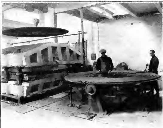
Garden hose mould being filled with 500 feet of uncured hose preparatory to vulcanization. In the press shown at the left another 500-foot length of hose is being cured at the same time.
