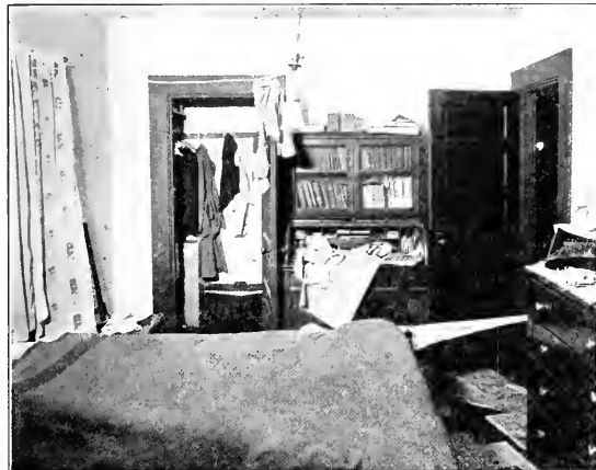
A typical incendiary. Practically everything in this room was saturated with kerosene. Note the cloth stretched from dresser to bed to carry the flame.
